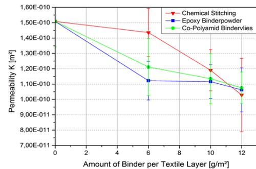
Figure 3: Permeability depending on binder system at 0° fiber orientation
