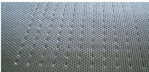
Figure 2: Preform locally fixed by using "Chemical Stitching" approach
